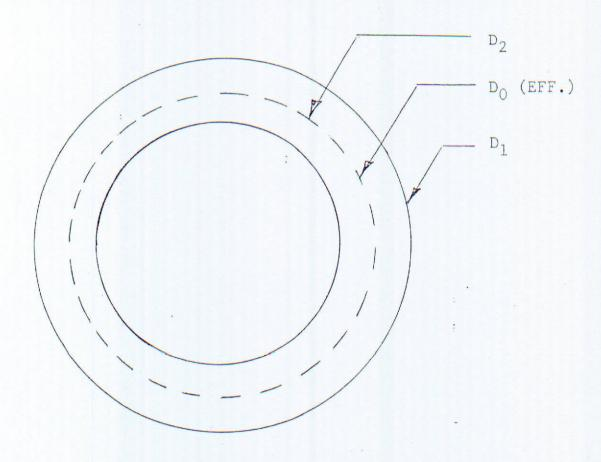
D<sub>2</sub> --- GUARD RING I.D. OR MEASURING ELECTRODE O.D. (COATED, TEFLON)
